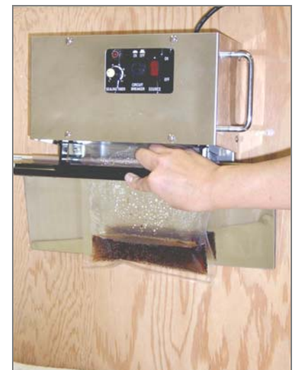
Sealing liquid with vertical sealing.
